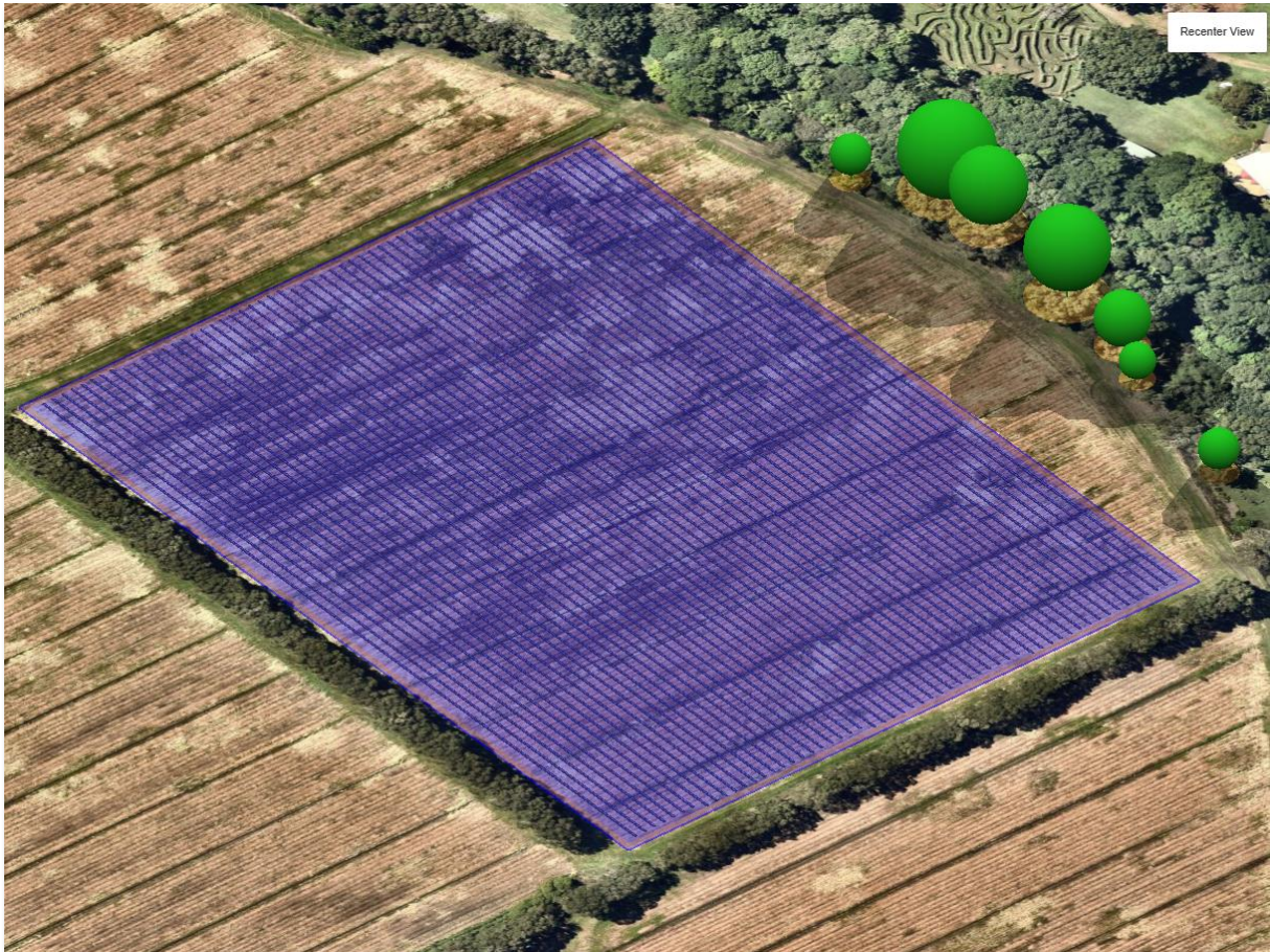
FIGURE 39: ROUS COUNTY COUNCIL'S LAYOUT OF A 2.7-MW SOLAR FARM AT GALLANS RD ESTATE
